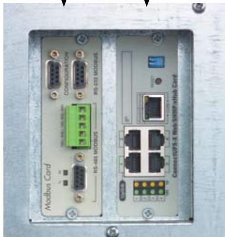
Two standard, embedded communication bays provide “plug-and-play” support for multiple communication cards. A total of four communication bays are available with the communication expansion option.
